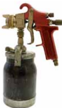
Figure 8.12: Paint guns spray paint more evenly than paint spray cans
